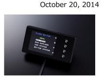
HKS' ECU ReFlash tool is available for tuning beginners and professionals. Flash Editor is a setting tool for ECU reflash via OBD II connection.
